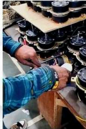
Motor H V Testing
